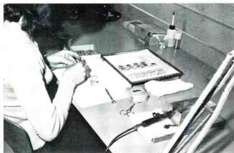
Studer makes most record and play heads for his machine. Here, assembly of one-inch heads.
