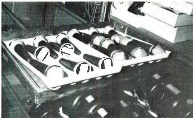
M-500s all in a row, awaiting only their top protective cover and a final q.c. before packing.
