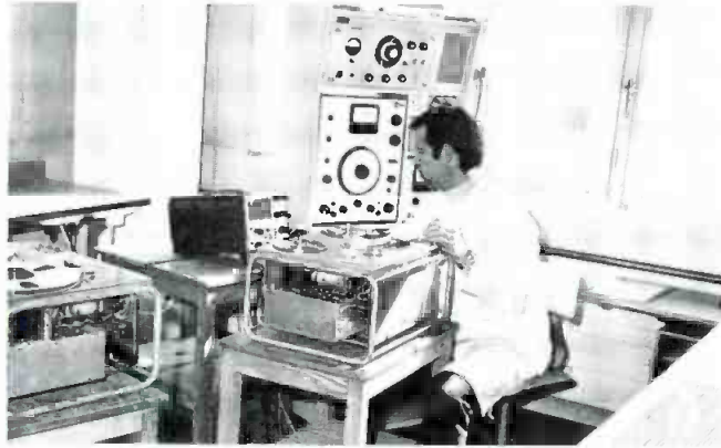
Studer B-62 units are still a big part of production. Here a completed one undergoes final adjustment.
