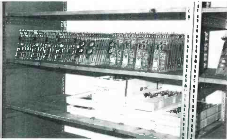
Circuit boards for A-80s are preassembled and stacked for later plug in to finished units.
