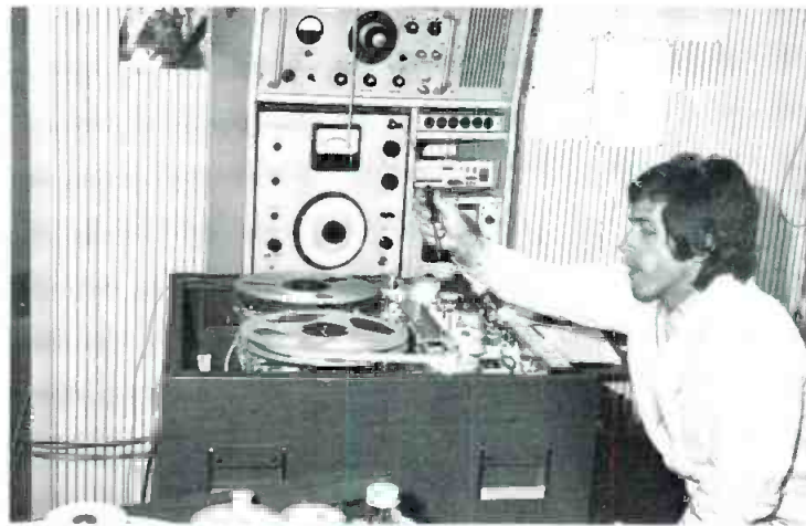
Final test and adjustment of A-80 machines. Test is a critical part of assembly taken most seriously at Studer.
