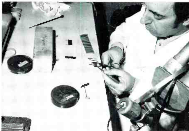
Thin metal strips are cut and placed in a pressure jig that forms them into precise ribbon elements.
