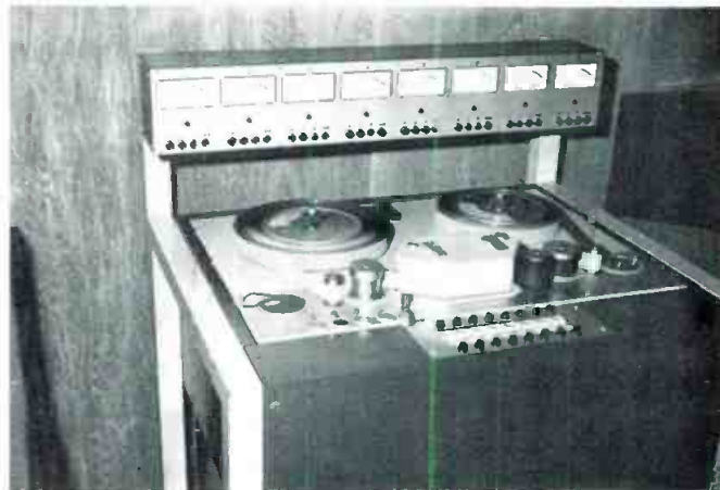
Philips Pro 72 is an eight track one-inch machine that is available in the U.S.
