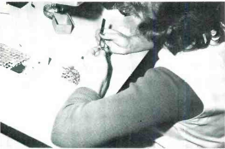
The pre-formed wire coils for transformers undergo lamination assembly here.
