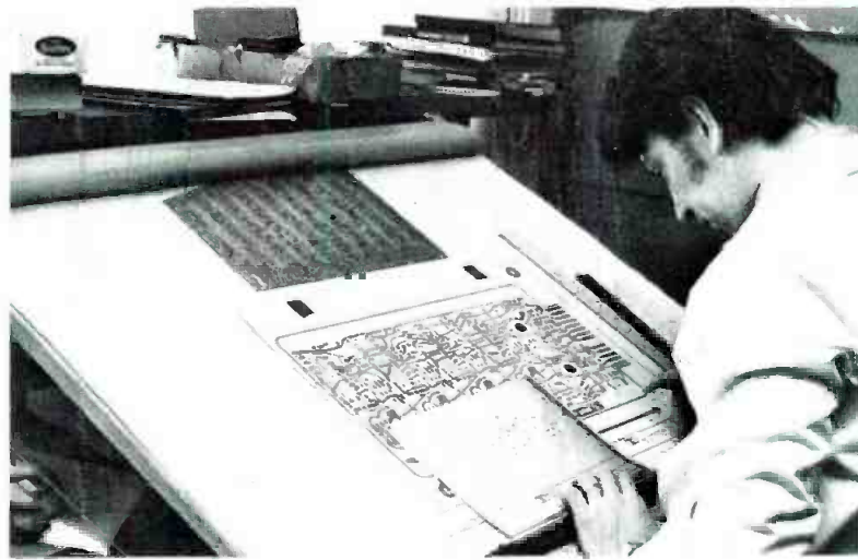
A drafting department is kept busy on new circuits—here a p.c. board layout is being created.
