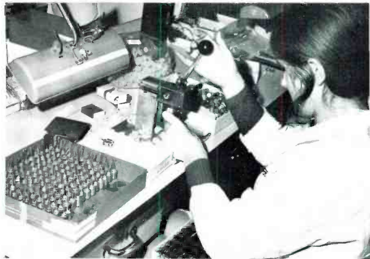
Finally, the completed transformer assembly is inserted and sealed in a metal case.
