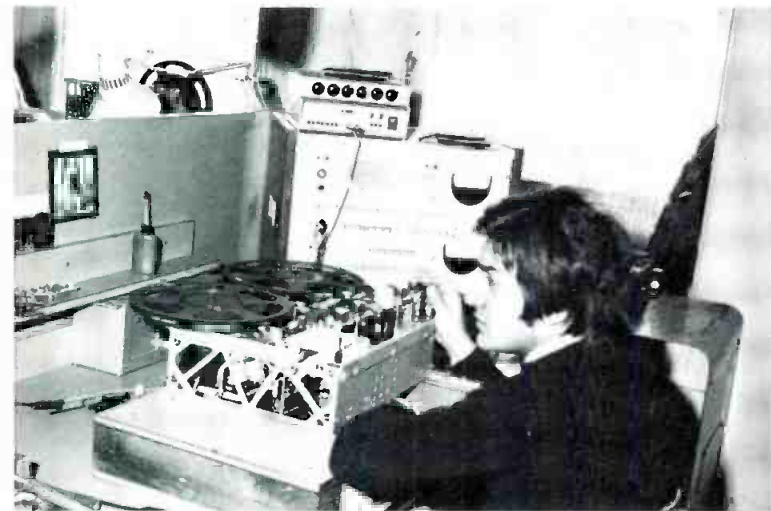
Test and adjustment of finished A-77s. Test and retest is an important part of production.
