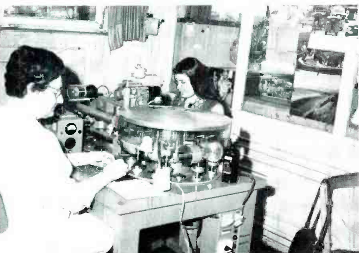
This machine automatically winds the correct amount of wire for a transformer onto a coil former.
