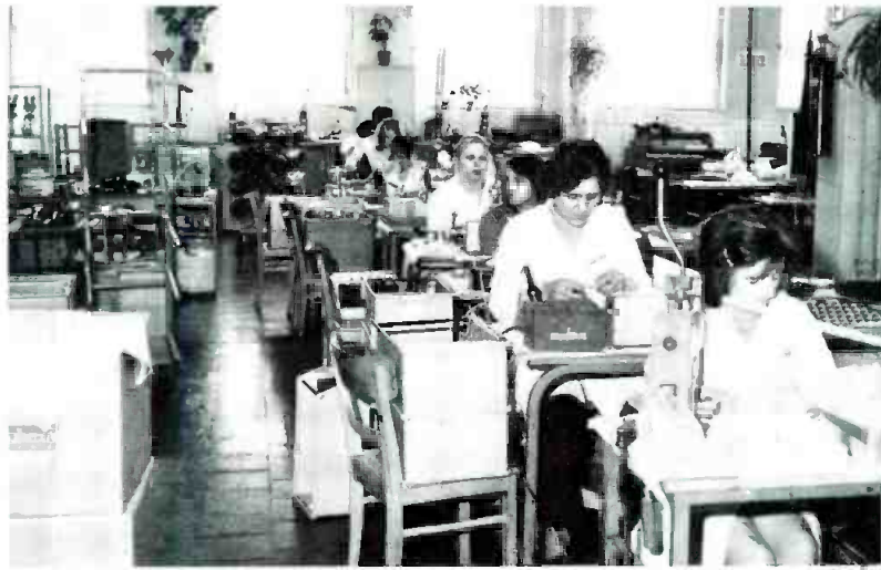
This typical small production line assembles small parts for insertion later into a microphone, transformer case, or headphone.
