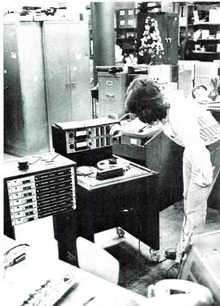
An Ampex AG 440 and Dolby equipment being checked and aligned prior to shipment.
