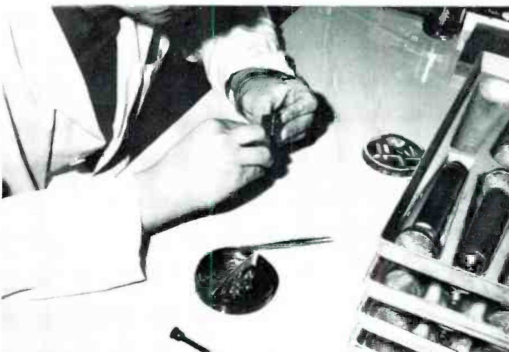
The cup in the foreground holds formed ribbons, the hands install one in an M-500 holder.
