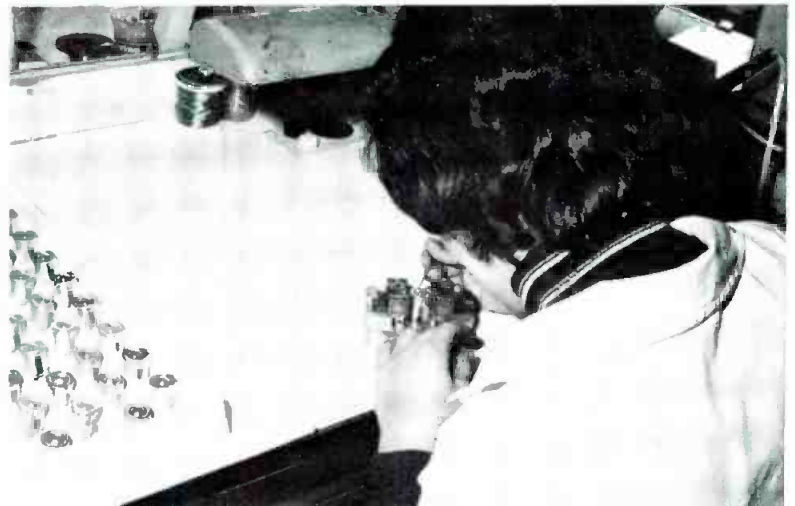
Delicate hand operations seal the diaphragm for a moving coil microphone.
