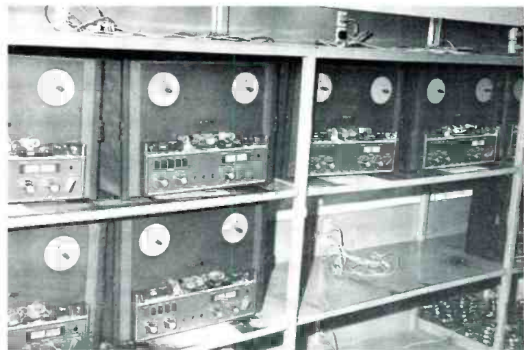
Finished A-77 units are run in and cycled on and off on this special jig.
