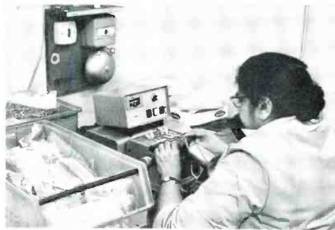
Lead cutting of resistors and diodes are done on this equipment. The performed result is ready to go into an appropriate place on a circuit board. Dolby uses over 50,000 resistors alone per week in his production.
