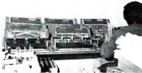
Dress panels for ReVox A-77s are checked and pre-assembled at this station.
